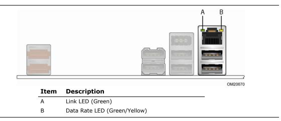
Figure 5. LAN Connector LED Locations
